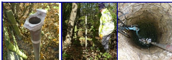
Piezometers and Well Monitoring at Stonehenge Farm
