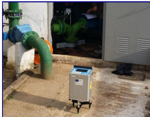
Microgravity Data Acquisition with a Scintrex CG-5 during an aquifer test at source Abstraction Borehole
